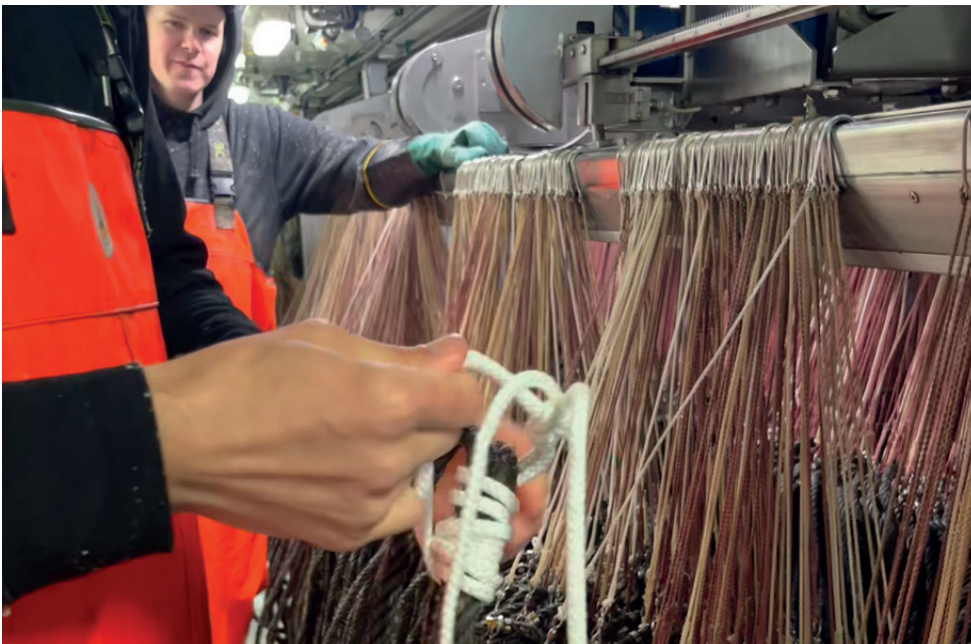
Testing of 6mm wood fiber ropes to connect the line sections on board MV "Loran". Photo: Anja Alvestad, SINTEF Ocean.
