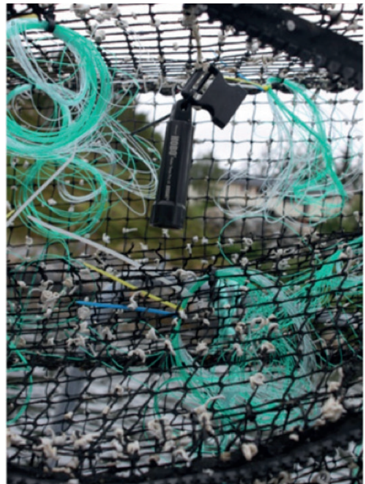
Fig. 1: Temperature logger and monofilament samples fixed in a pot.
