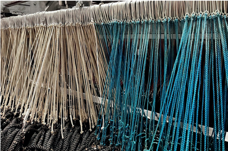
Experimental set-up on board the autoliner MV "Loran" – biodegradable snoods in white, and conventional snoods in blue. Photo: Anja Alvestad, SINTEF Ocean.
