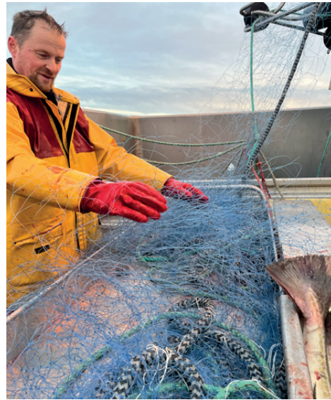
Work on board MV "Karoline": Fish caught with traditional nylon gillnets (green, left) and biodegradable gillnets (blue, right). Photo: Jørgen Vollstad, SINTEF Ocean
