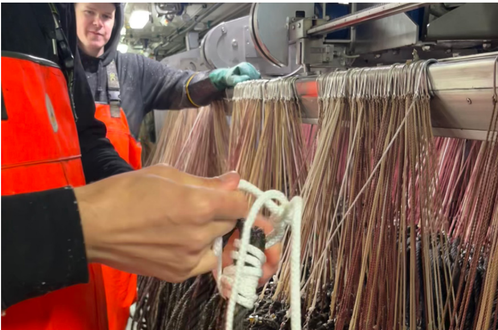
Testing of 6mm wood fiber ropes to connect the line sections on board MV "Loran".
