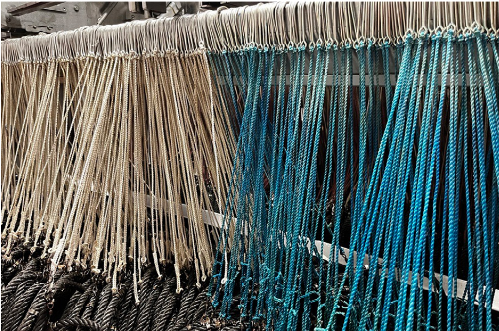
Experimental set-up on board the autoliner MV "Loran" – biodegradable snoods in white, and conventional snoods in blue.
