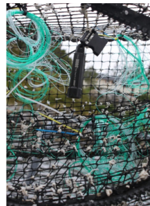
Temperature logger and monofilament samples fixed in a pot. Photo: SINTEF Ocean
