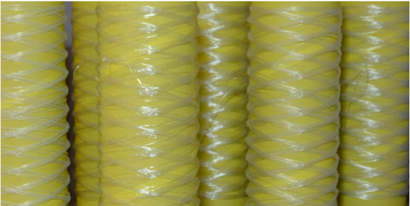
Monofilaments produced from different bioplastics materials in the Dsolve project.
