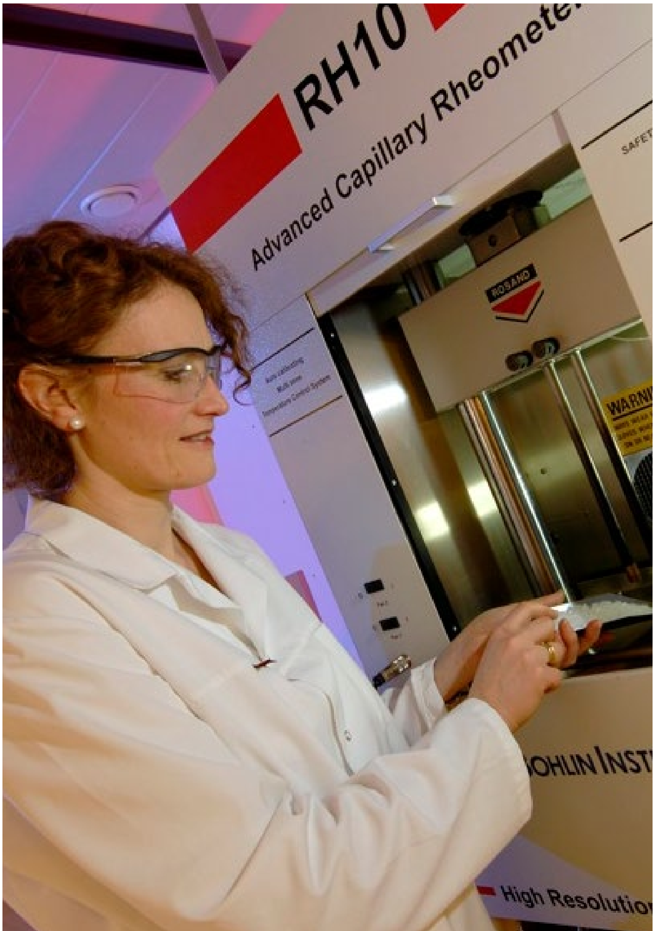
Capillary rheometer (Haul-off) to determine melt strength and melt spinnability. Photo: Norner Research
